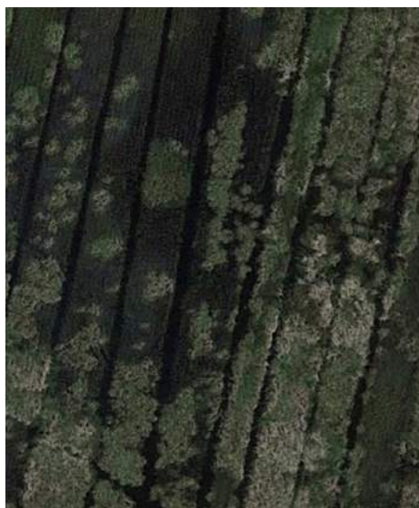
Quarter Drains in Combahee River Rice Field. These parallel, shallow ditches facilitate water circulation and de-watering of historic rice fields
